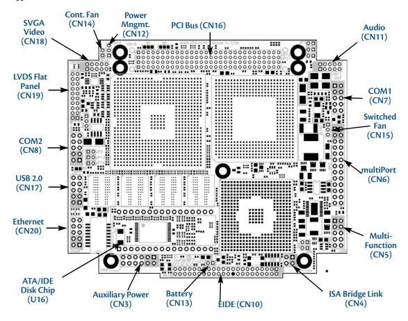
Figure 1 CMX158886 cpuModule (top view)
